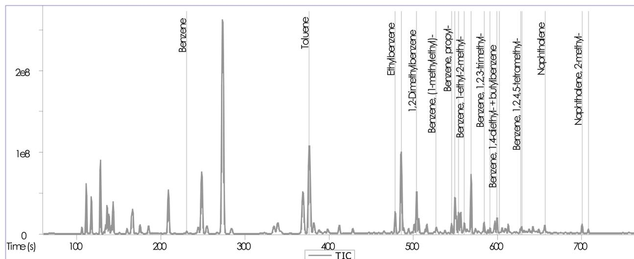
Figure 3: A total ion chromatogram (TIC) of 93-octane commercial gasoline is shown above with peak markers automatically placed for the 23 calibrated analytes. The table below reports concentration values for both calibrated and uncalibrated analytes of interest in volume % as specified in the method.
