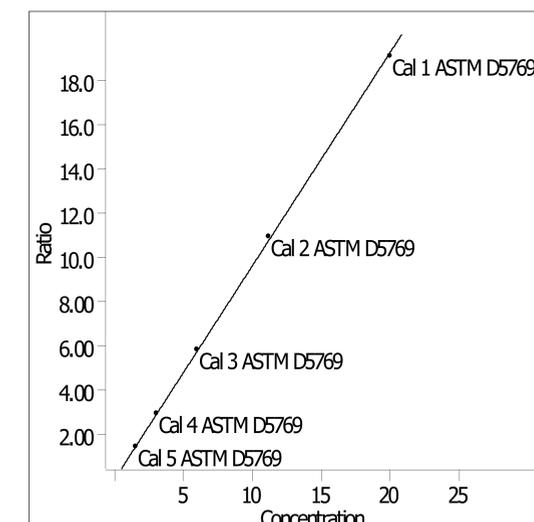
Figure 4: The calibration curve for toluene illustrates the excellent linearity that is shown in the table of R<sup>2</sup> values for each calibrated analyte.
