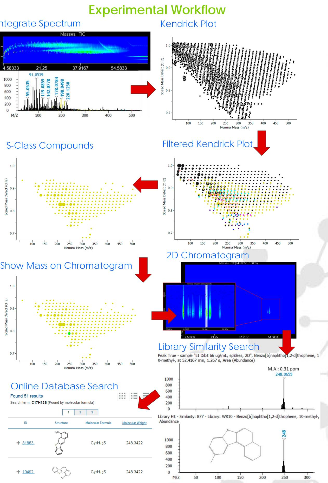
Comprehensive two-dimensional GC coupled to HRTOFMS is a powerful tool for chemical characterization. This technique is ideal for petroleomics because it provides mass determination, heteroatom class, type, and carbon number information similar to direct high resolution mass spectrometry, and additionally gives well-defined chromatographic regions that facilitate structural elucidation and speciation.
