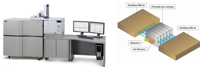
Figure 2. LECO's Pegasus® HRT and FFP™ Mass Analyzer.
