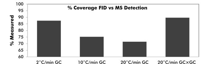
Figure 5. Relative Coverage of FID vs. MS. The number of peaks detected with FID/number of peaks with MS is shown for each method. Of note, the GC×GC separation had a greater total number of detected analytes, so some coelutions result from the ability to detect additional analytes.
