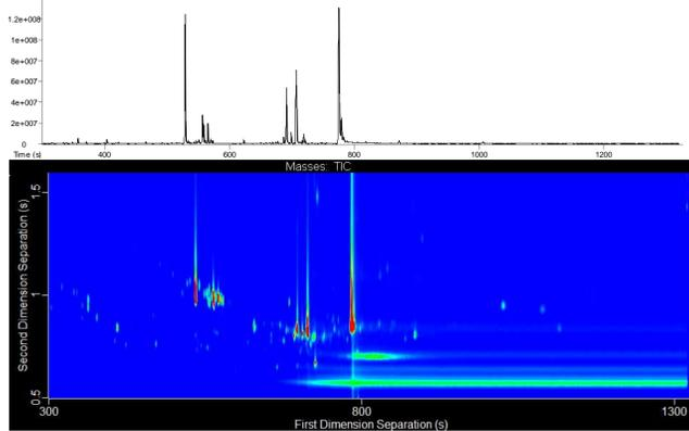
Figure 2. GC and GC×GC separations of Blue German Chamomile. Many coelutions in the GC separation were chromatographically resolved in the second dimension without increasing the analysis time.
