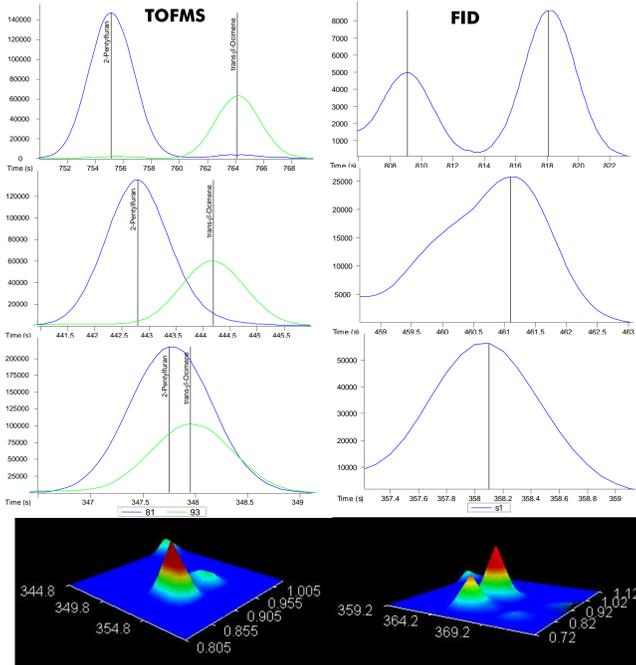
Figure 3. 2-pentyl furan (m/z 81) and trans-β-ocimene (m/z 93) are baseline resolved with a two-hour separation, but are indistinguishable by FID in the 22-minute separation. With GC×GC, this near-complete coelution in the primary dimension is baseline resolved in the second dimension presenting no problems for identification or quantification.
