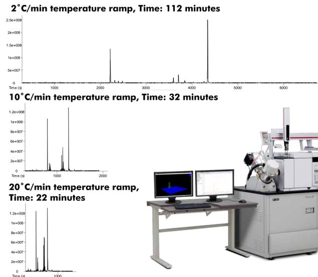
Figure 1. Blue German Essential Oil. Representative TIC chromatograms show the impact of faster temperature ramp rates.
