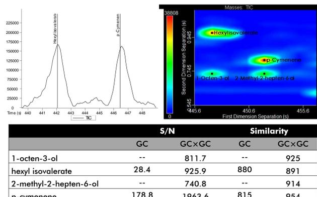
Figure 4. Additional analytes were detected with GC×GC relative to GC, in part due to thermal focusing at the modulator.
