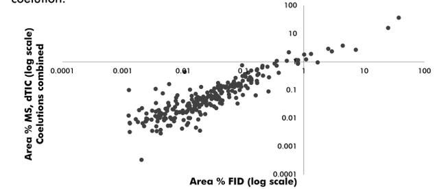
Figure 6. Area % FID vs. TOFMS. This correlation ( $R^2 > 0.95$ ) suggests that dTIC Area % information with TOFMS deconvolution may complement and supplement FID Area % in cases of coelution.
