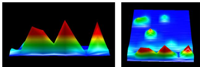
Figure 2. GCxGC increases the peak capacity relative to a 1D separation. (Standard sample shown.)
