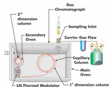
Figure 1. Diagram of the major GCxGC components.
