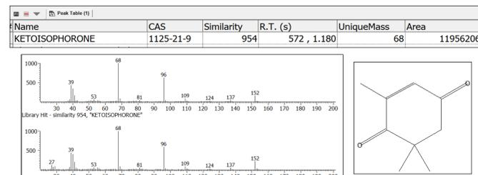
Figure 4. Representative analyte information provided by ChromaTOF's automated peak finding software. Ketoisophorone was identified in all samples.
