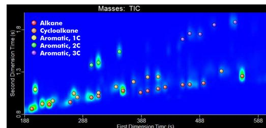
Figure 3. Analytes with similar functional groups elute in structured bands through the GCxGC space. (Standard sample shown.)
